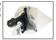
**8b** Chamfer end of pipe using <u>Continental's</u> double ended <u>ID chamfering</u> tool.
