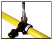
**9** Mark the stab depth by inserting pipe into ID chamfer tool and marking the pipe at the entrance as shown.
