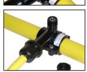
11 Stab pipe completely into outlet so that the stab depth mark on the pipe is within 1/8" from the fitting entrance.
