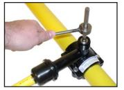
10 If using ID chamfer tool with gauge, check for proper chamfer by inserting pipe on gauge up to the o ring. With proper chamfer, o ring will begin to enter pipe.
